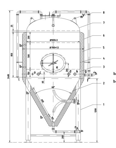
Technical parameters 1.The inner surface polished to Ra ≤ 0.22 μm. 2.Outer surface adapts high accuracy Polishing. 3.Nozzle position by vertical view. 4.To filled with water in tank for leak testing.
